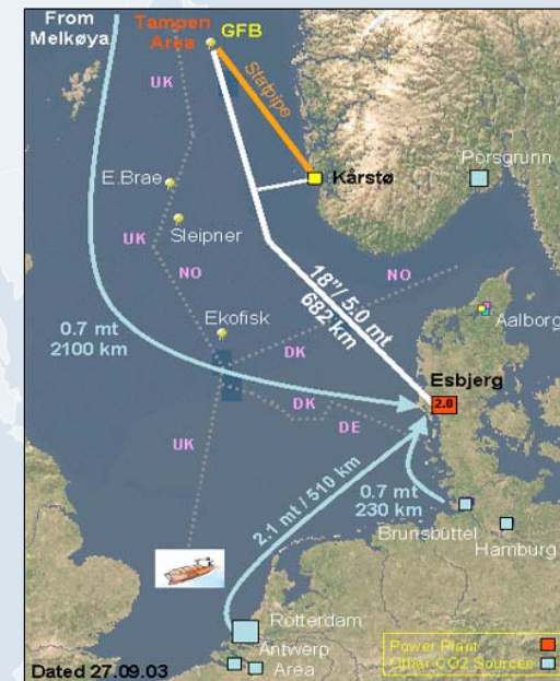
A network of sources and transportation means to supply Gullfaks with 5.5 MT CO 2 /year. From Elsam (2003)
